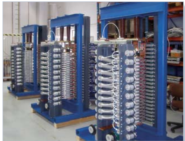
SVC for Danieli, Italy. Factory tests at Nokian Capacitors
