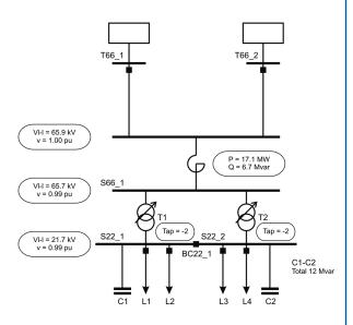
Improving the power factor of the zone substation load to 0.93 or better results in excellent voltage regulation and allows the system to operate with the tapping range of the transformer. The 22 kV busbar voltage is improved to 0.99 p.u. and the transformer taps are at position -2.
