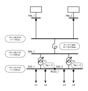
The two zone substation transformers have on-load tap changers configured to maintain the voltage of the 22 kV busbar within a narrow range.
