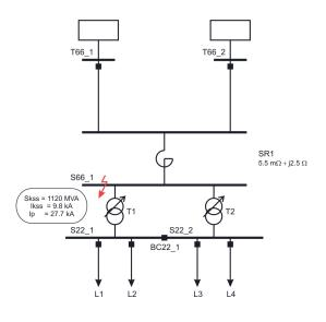
Placing a 2.5  $\Omega$  reactance in series with both feeders results in fault current of 9.8 kA, well within limits. The goal of additional power capacity and restricted fault current is therefore achieved with the combination of a new feeder and a series reactor.
