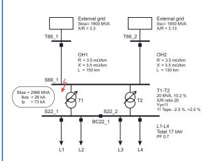
When the second 66 kV feeder is connected as shown, the fault level at S66\_1 increases to 26 kA, well over the rated value. Upgrading switchgear, cabling, busbars and other primary equipment to the higher fault level is time consuming and expensive.
