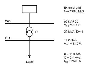
Assume that distortion at the PCC and plant busbar should be less than 1% and 3 % respectively. A two-stage harmonic filter tuned to the fifth and seventh harmonics is implemented to improve the situation.
