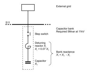
The total bank reactance can be calculated from the nominal reactive power requirement of the bank at nominal voltage,  $X_{\tau} = V_N^2/Q_N$ . This value and the relationships indicated in the figure above result in values of capacitance 122.3  $\mu$ F and inductance of 5.8 mH.
